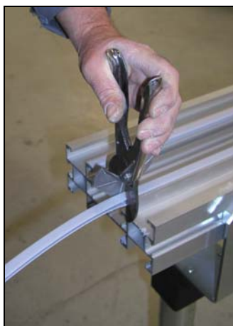
Cut the end of the sliding gib at right angles
