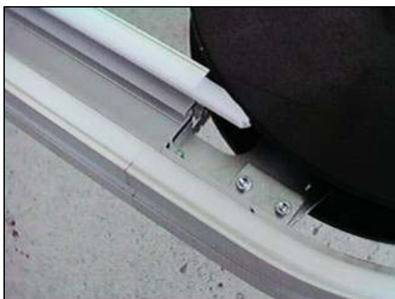
Sliding gib must be trimmed to fit the shape of the bend wheel
