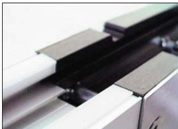
Sliding gib must be cut to be flush with the drive station
