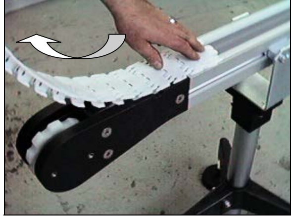
Disassembly of the link chain
