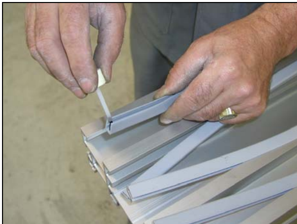
Each sliding grib must be fixed at the beginning (as viewed in running direction)
